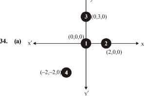
$I_1 = I_2 = 0$ , because these particles are placed on x-axis The M.I. of system about x-axis,  $= I_1 + I_2 + I_3 + I_4$  $= 0 + 0 + 3 \times (3)^2 + 4 \times (-2)^2 = 27 + 16 = 43 \text{ kg} - \text{m}^2$
