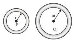
Moment of inertia of loop P,  $I_p = mr^2$ Moment of inertia of loop Q,  $I_Q = nm(nr)^2 = n^3mr^2$
